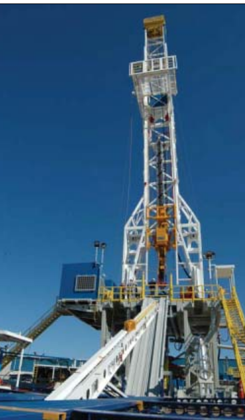
Nabor's M-series rigs (left photo) can operate on locations with limited space (Fig. 2). One feature on the PACE rigs (middle photo) is an automated iron roughneck (Fig. 3). The PACE rigs (right photo) have automated catwalk pipe handling systems (Fig. 4).
