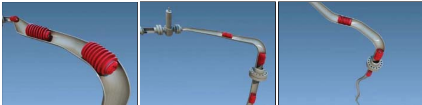
The topside pipeworks shown here (left photo) are not traditionally pigged, requiring pigging for the low-pressure isolation through nonstandard construction pipework fittings (Fig. 2). The nonstandard construction pipework fittings (middle photo) consisted of two 1.5-D bends and a narrow 45° traverse (Fig. 3). The geometry of the damaged section (right photo) of riser was unknown, requiring emphasis on maintaining the section's integrity while running the pig train through the riser (Fig. 4).
