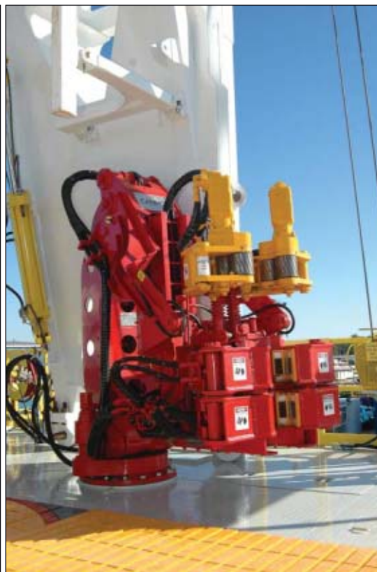
Nabor's M-series rigs (left photo) can operate on locations with limited space (Fig. 2). One feature on the PACE rigs (middle photo) is an automated iron roughneck (Fig. 3). The PACE rigs (right photo) have automated catwalk pipe handling systems (Fig. 4).
