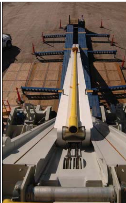
Nabor's M-series rigs (left photo) can operate on locations with limited space (Fig. 2). One feature on the PACE rigs (middle photo) is an automated iron roughneck (Fig. 3). The PACE rigs (right photo) have automated catwalk pipe handling systems (Fig. 4).
